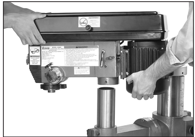
Figure 10. Mounting the headstock.
